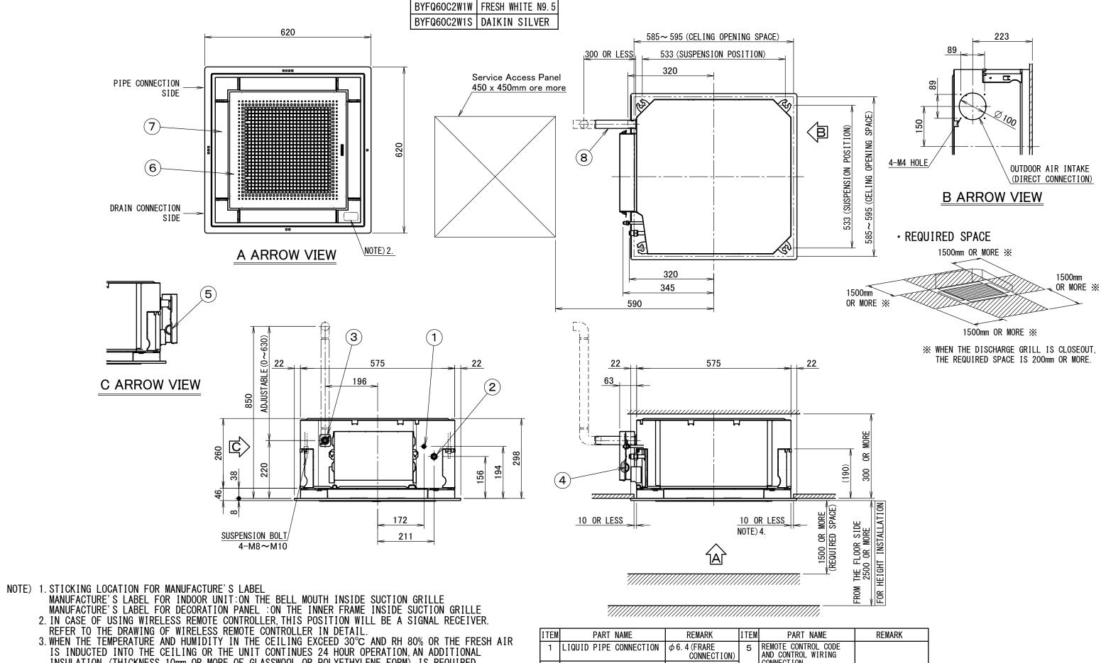
INSULATION (THICKNESS 10mm OR MORE OF GLASSWOOL OR POLYETHYLENE FORM) IS REQUIRED.
