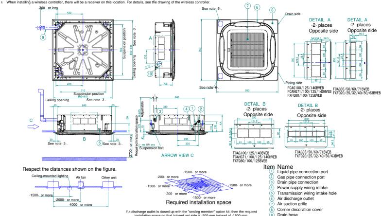
installation space on that (closed up) side is .500 mm instead of .1500 mm.
