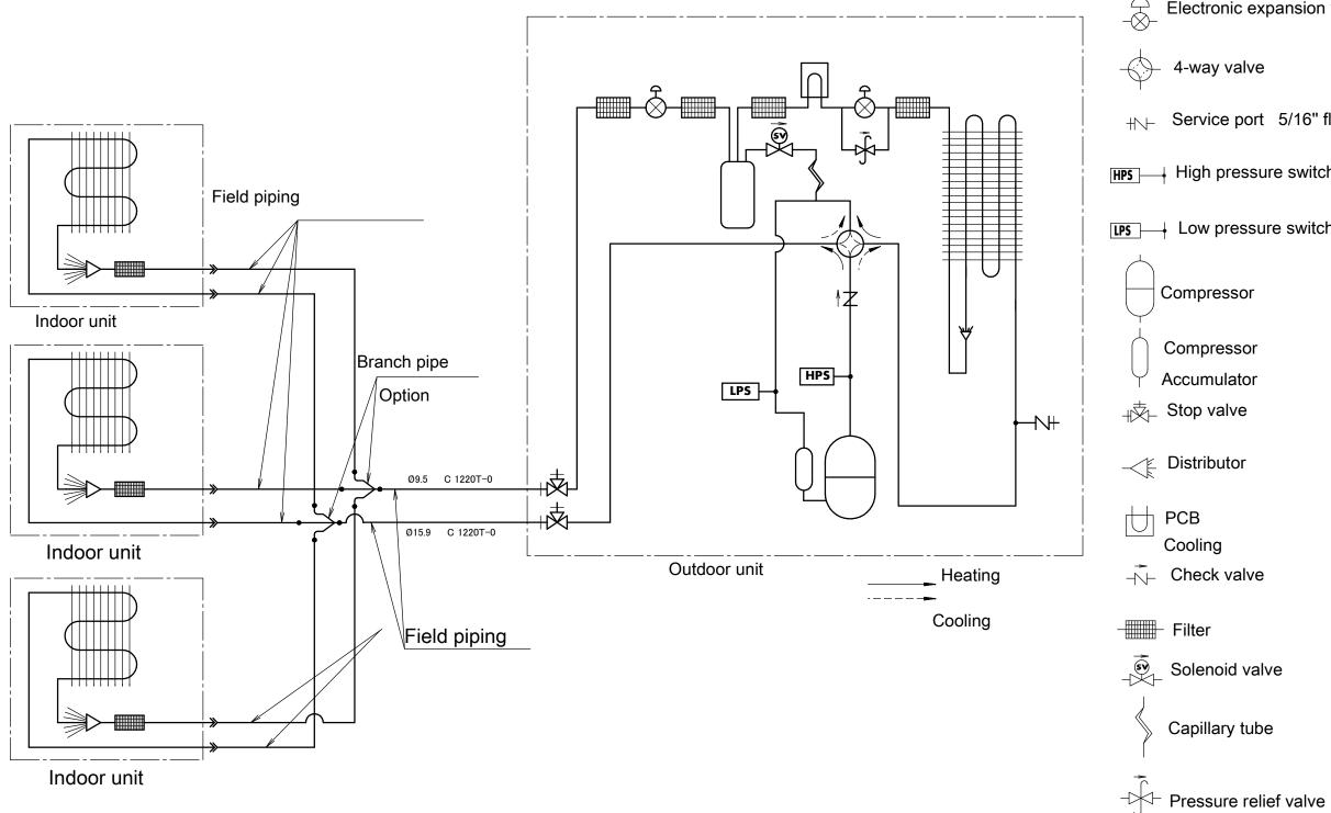
Liquid receiver Heat exchanger Electronic expansion valve 4-way valve Service port 5/16" flare High pressure switch Low pressure switch Compressor Compressor Accumulator Stop valve
